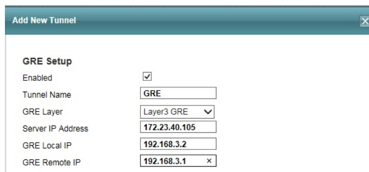
Figure 14-6 Layer 3 GRE VPN Configuration Example, Add/Edit GRE Tunnel
